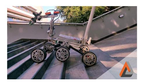
Anveshak performed exceptionally well in the Extreme Retrieval and Delivery Task, and were able to test the capabilities of their new modified Carbon Fibre Rocker-Bogie Mechanism, scoring 96/100.
